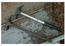
tops. The hammers were run up to 1600F, oil quenched, and tempered at 600F for an hour. That makes them resilient but softer than a normal hammer. Extra long handles were welded, and we were good to go. The process consisted of slipping the claws of the modified hammer around a nail head, whacking the face with a normal 2 lb framing hammer, and popping the nail free. It took two of us approximately 6 hours to strip the 1500 ft<sup>2</sup> oof and there was
